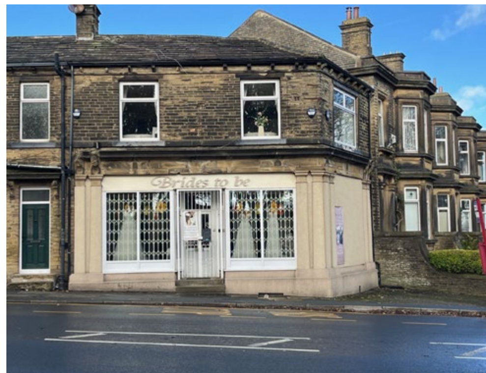
Brides to be, Scarlet Heights, Queensbury – The internal concertina grilles allow for views of the goods when closed and can be neatly tucked away inside the window jams when open
